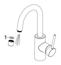
After installing faucet, remove aerator. Turn water on for 30 seconds to remove any debris. Reassemble aerator. Do not lose the gasket (1) in the aerator.
