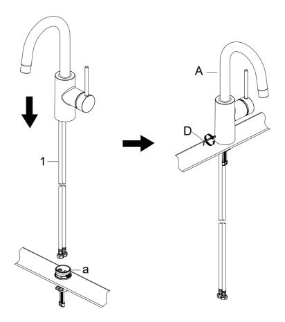
Insert the supply lines (1) through the hole of the base (a). Carefully insert the hoses into the base. Place the faucet assembly (A) onto the base (a) as shown in the above figure. Secure the faucet assembly (A) by tightening the set screw with the provided hex wrench (D, Hex: 2.5 mm).
